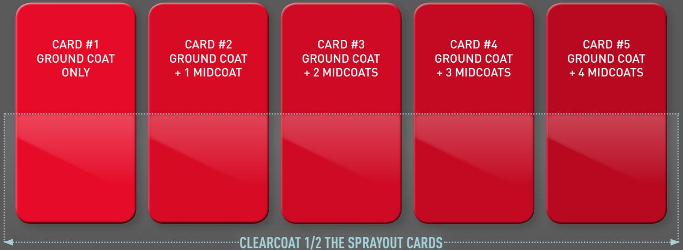
CREATING A LET-DOWN TOOL WILL VERIFY THE NUMBER OF MIDCOAT LAYERS REQUIRED FOR THE TRI-COAT VEHICLE COLOR BEING REPAIRED.
